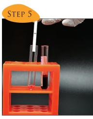
INSERT THE MEMBRANE INTO THE WELL TO ALLOW THE MIGRATION.
