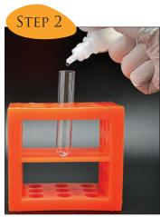
ADD 3 DROPS OF BUFFER INTO THE CLEAN TEST TUBE.
